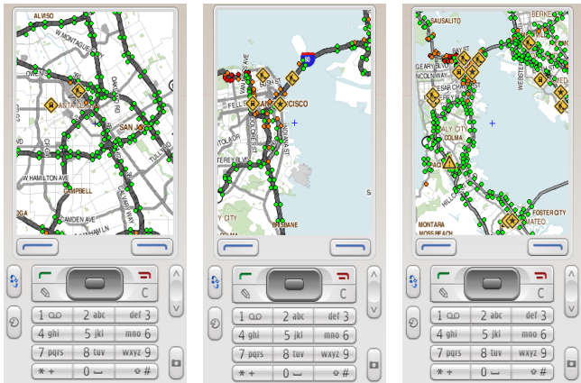
Fig. 3. Nokia N95 client emulator used for development of our system. The client serves both to collect data from individual devices, and to display current traffic conditions. The colors in the circles represent the speed of traffic (green corresponds to free flow; red is congested). (Left) Free flowing traffic in Santa Clara, CA. (Middle) Congestion occurs in San Francisco, CA. (Right) Bay Area regional traffic.
