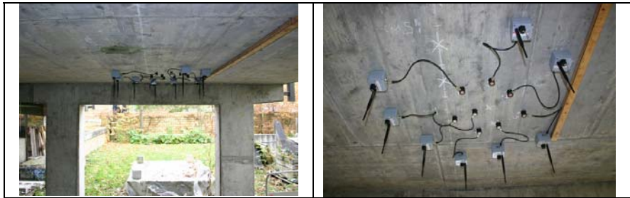
Fig. 5 Overview of setup for wireless AE measurements at the Stuttgart “ramp” (left) and wireless AE array setup (right)
