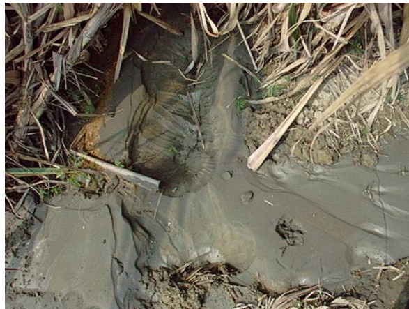
Figure 2 Sand boils in a rice field at Jingliao following the Chiayi earthquake
