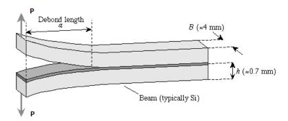
Figure 1: A double cantilever beam
