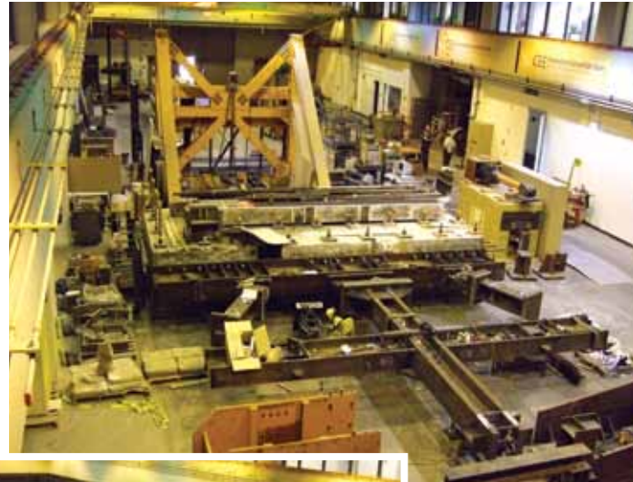
Above: West end of the laboratory showing a test setup for a full-scale steel beam-column joint. Left: East end of the laboratory showing construction of full-scale reinforced concrete beam specimens.
