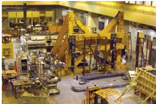
Above: West end of the laboratory showing a test setup for a full-scale steel beam-column joint. Left: East end of the laboratory showing construction of full-scale reinforced concrete beam specimens.
