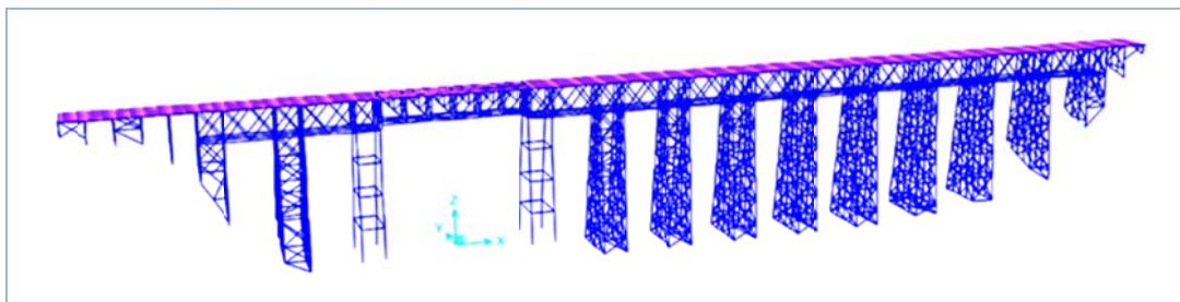
Figure 12: Analysis model of the Albion River Bridge
