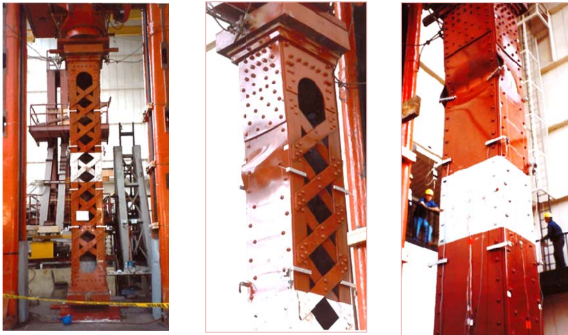
Figure 5: Truss chord specimen and its local buckling during the test [7]
