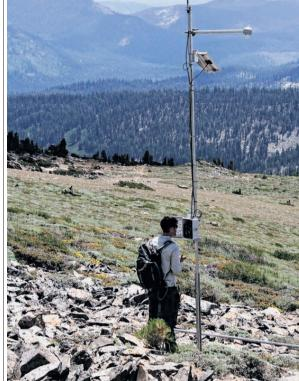
ember of Professor Steven Glaser's team from UC Berkeley makes notations about one of the sensor will help measure the state's water supply while recording temperature, relative humidity and more
