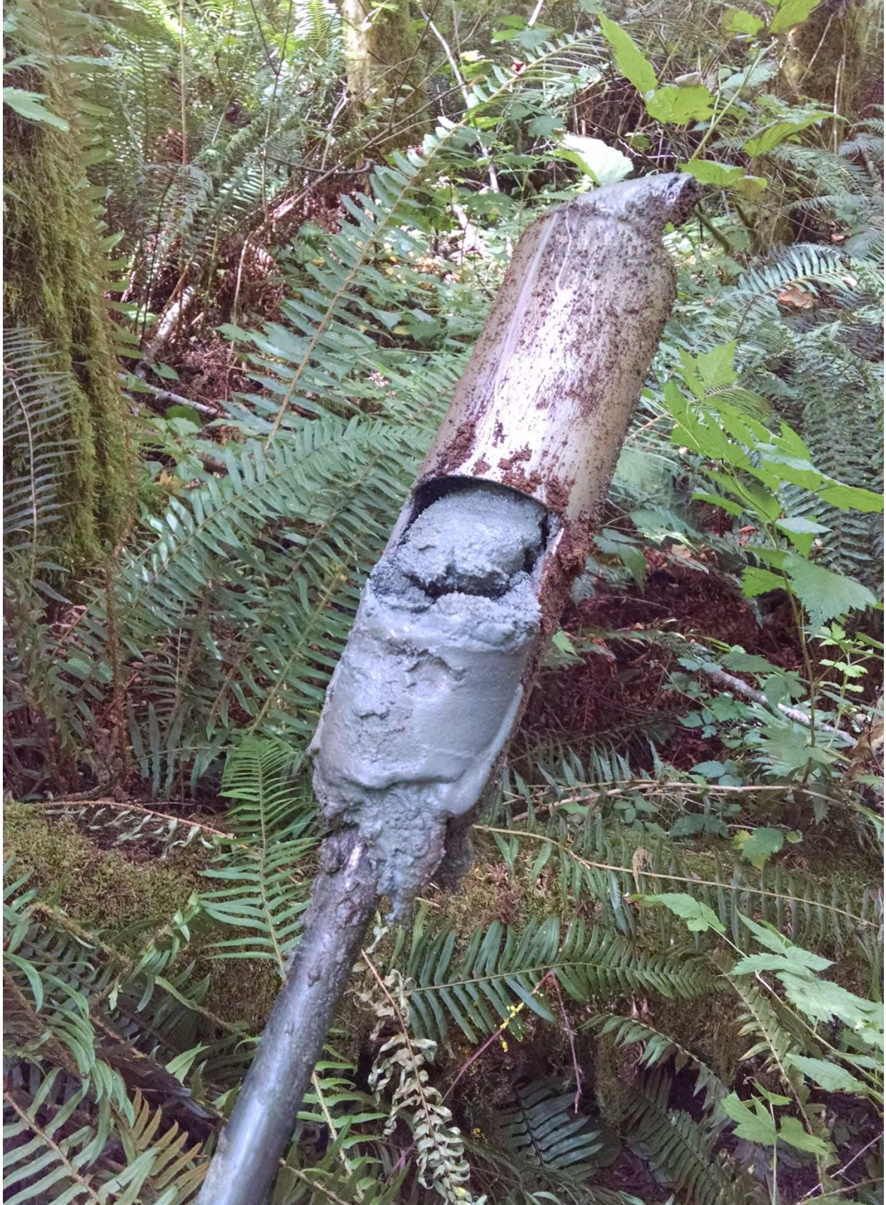
Figure 14: Hand auger within Headache Creek encountered sandy clay (location #2 in Figure 12).
