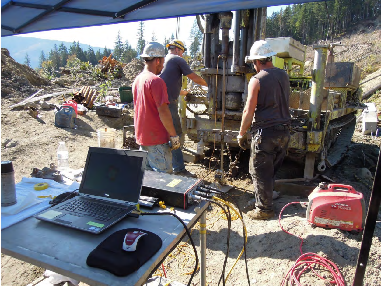
Figure 11: Pushing CPT with the CME-850 at the EB-12 exploratory location.
