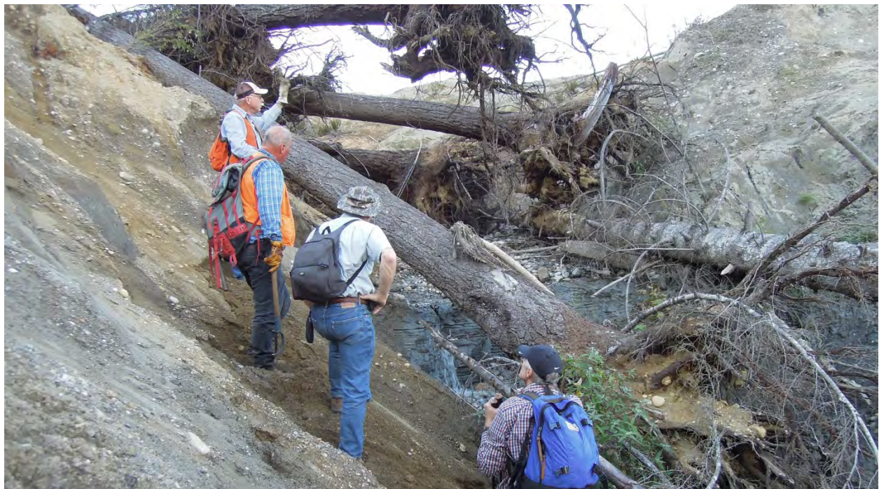
5 6 Figure 10: View of glacio-lacustrine silt and clay exposure of surface of rupture (photo taken 10/23/2015 at 7 48.282N; 121.848W, looking N).
