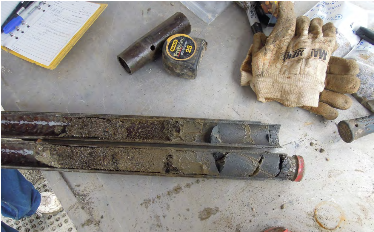
12 13 Figure 8: Surface of rupture delineated at contact of recessional sand and glacio-lacustrine silt and clay at boring 14 EB-04-si-15.
