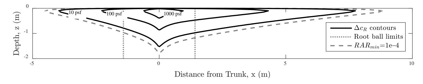
Root reinforcement (effective cohesion) for a surveyed levee slope, comparing 3D sliding surfaces and estimated lateral root limits:
