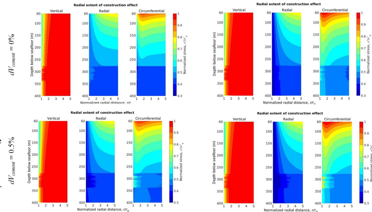
The effect of cement shrinkage can be seen in the contour maps. They show stress distributions around the wellbore with 0% (top) and 0.5% (bottom) cement volume shrinkage. The stress disturbance was aggravated by cement shrinkage. Also, smaller cement slurry density enlarged the zone of influence of wellbore construction.
