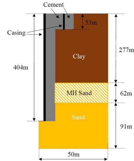
Geometry of the finite element model.
