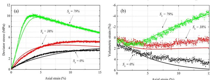
Critical state constitutive model: calibration result (the dots are the experimental data by Yoneda et al. (2015)).
