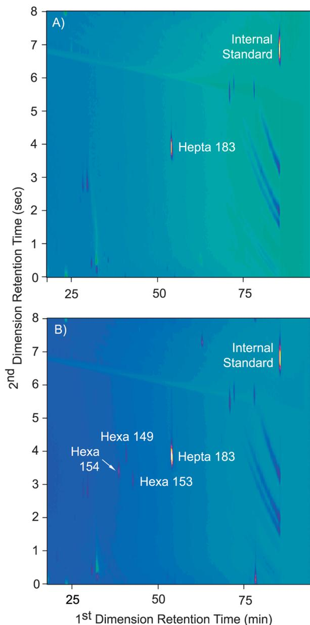
**FIGURE 2. Debromination of Hepta 183 by the ANAS195 culture. The GC  $\times$  GC chromatograms show (A) the autoclaved control and (B) an active sample showing generation of various hexa-BDE congeners during debromination of Hepta-BDE 183 after 3 months.**
