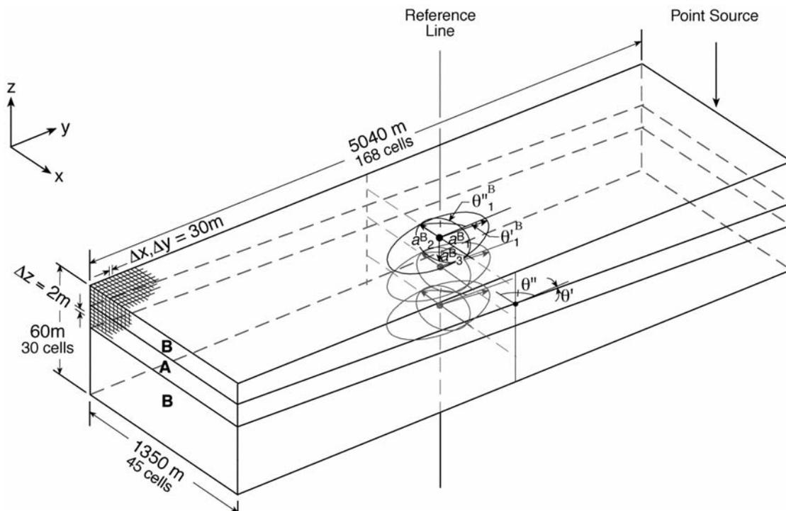
Fig. 9 Grid and parameters for indicator simulation. From Ritzi *et al.* (2000).
