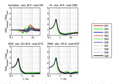
FIG. 8. Pseudo-acceleration floor response spectra of the isolated structure normalized to the respective spectrum of the non-isolated structure (median spectra; X direction)
