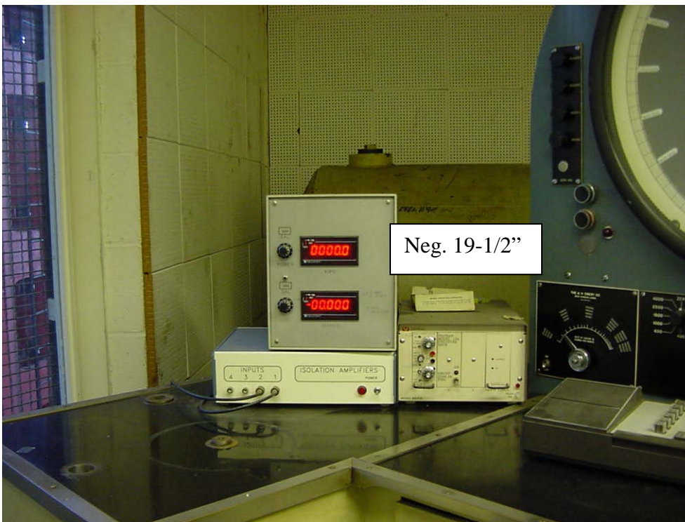
11. Retract screws 48" meter reading minus 19-1/2" for a starting place.
