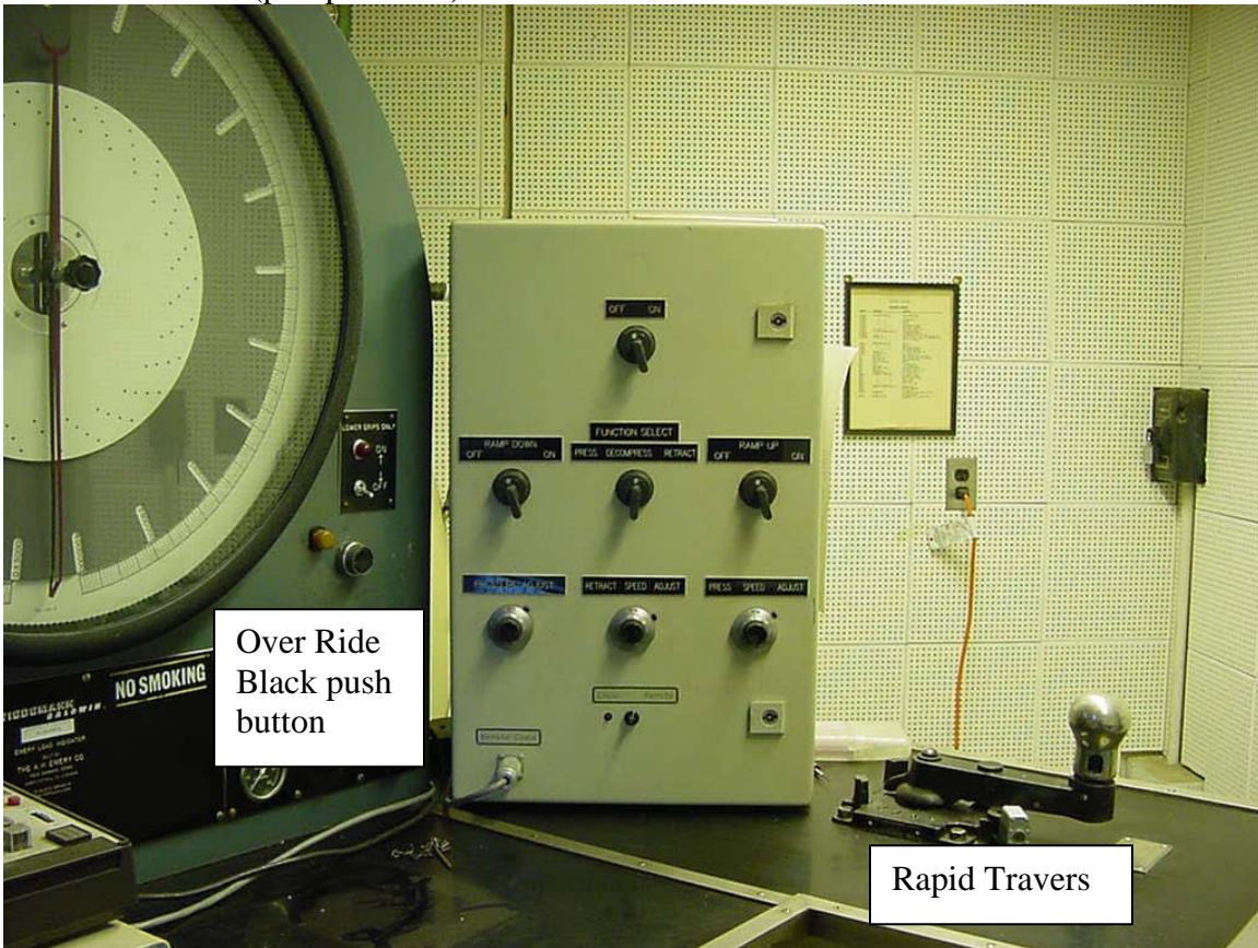
Adjust head with Rapid Travel, and turn Hydraulic Control Unit switch to "Return, or Press"
